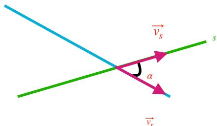
$$\cos \alpha = \frac{|\vec{v}_r \cdot \vec{v}_s|}{|\vec{v}_r| \cdot |\vec{v}_s|} = x \quad \rightarrow \quad \alpha = \arccos(x)$$
